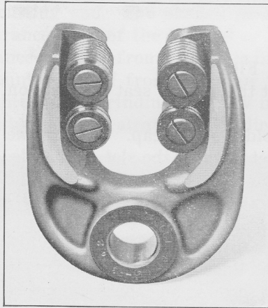
Fig. 10. Go-not go thread gage
